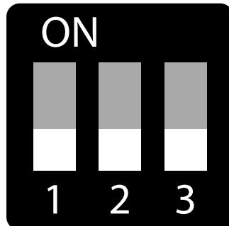
**1 DRY/BYPASS DIP SWITCH:** This switch is only active when the REAMP switch is set to the PWR AMP position. With PWR AMP selected, the DRY/BYPASS DIP switch modifies the BYPASS and DRY signal path to incorporate the pedal's PREAMP circuitry.
