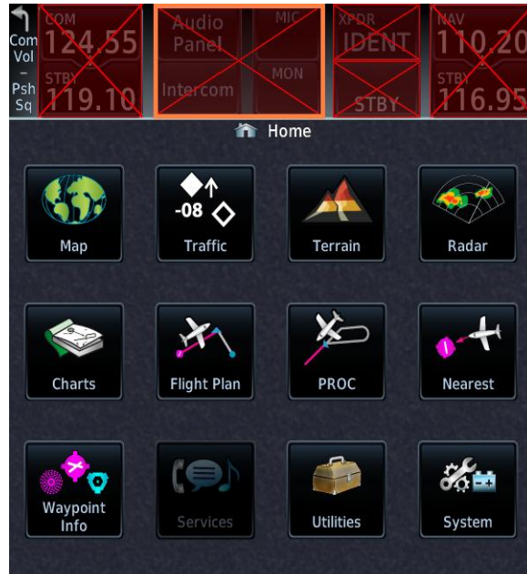
Figure 4-2 GMA 35 Failure Annunciation
