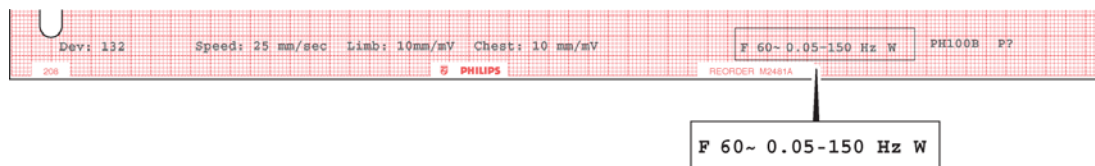
Figure 4-24 Filter Information Box on the Printed ECG Report
