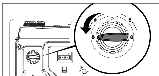
4. Move the choke lever to the "CHOKE" position.
