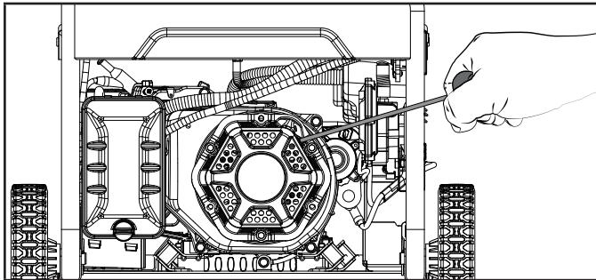
6. When engine starts running, move choke lever slowly to the "RUN" position over a 2-5 second period.
