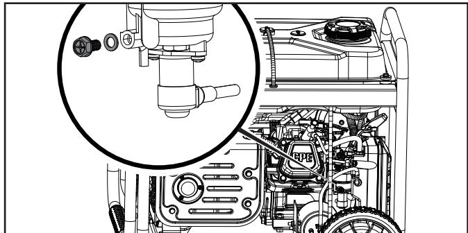
7. When gasoline stops flowing from the carburetor, replace and tighten the carburetor drain bolt and be sure to properly dispose of the drained gasoline according to local regulations or guidelines.
