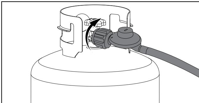
5. Open valve on LPG cylinder and check all connections for leaks by wetting the fittings with a solution of soap and water. Bubbles which appear or bubbles which grow indicate that a leak exists. If a leak exists at a fitting then turn off the valve on the cylinder and tighten the fitting. Turn the valve back on and recheck the fitting with the soap and water solution. If the leak continues or if the leak is not at a fitting then do not use the generator and contact customer service.
