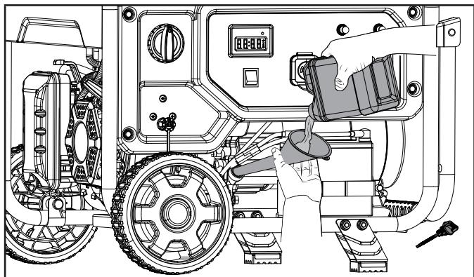
4. Check engine oil level at every use and add as needed.
