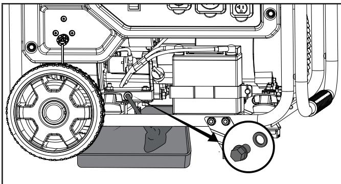
3. Replace the oil drain bolt.
