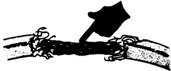
Figure 4-4. Belt Damage Due to Shock Load
