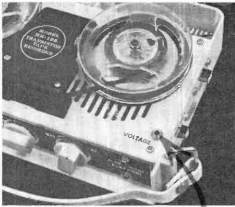
Subminiature jack (J2) for monitoring battery voltage can be installed on top of panel.
