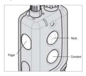
The transmitter for **dogtra1500NCP** has three buttons (two on the face of the transmitter and one on the side).
