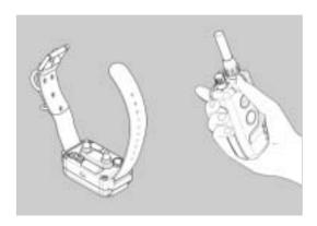
1. Turn the collar on by pressing the button on the back side of the collar receiver. The indicator light will come on for a moment then blink once every two seconds, showing that the collar is ready to use. (If the indicator light is red, the batteries need to be charged.) Place the test light on the contact points of receiver and hold it there.
