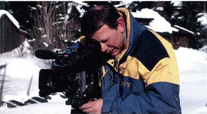
This camcorder, based on the Digital Betacam format, will be introduced in the summer of 1994. Through its introduction, a total digital system covering shooting, editing, and broadcasting will be made possible.
