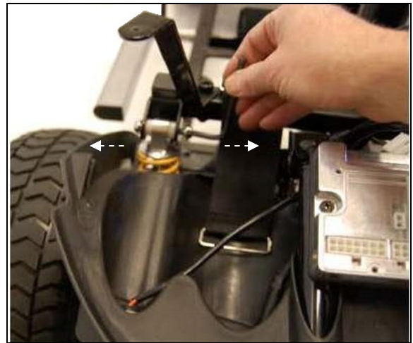
Figure 24. Shock Bolt Removal
