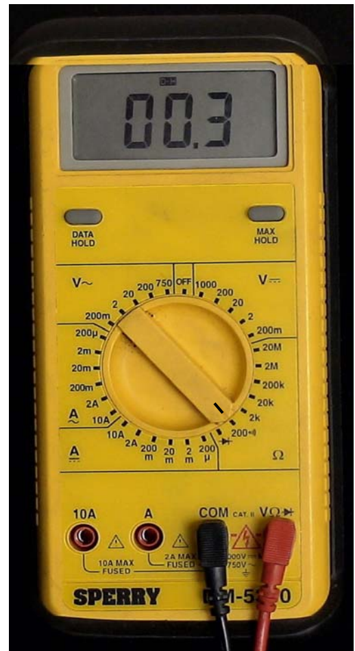
Figure 27. Multimeter (Set to Ohms)
