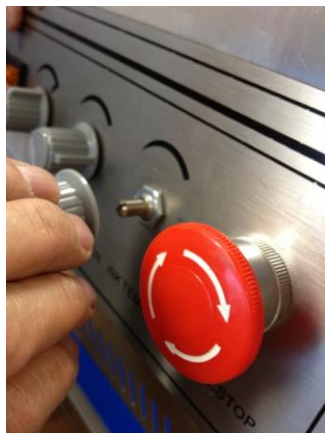
Figure 33. Remove Ink Temperature Knob
