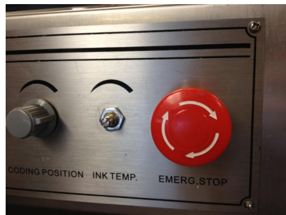
Figure 34. Remove Washer Holding Ink Temperature Potentiometer
