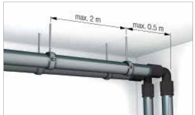
Fig. 7-8 Maximum pipe clamp intervals
