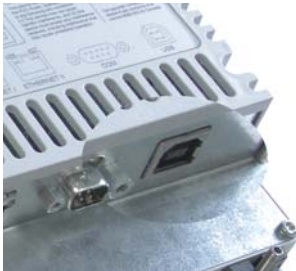
Figure 16: USB Device female connector Type B
