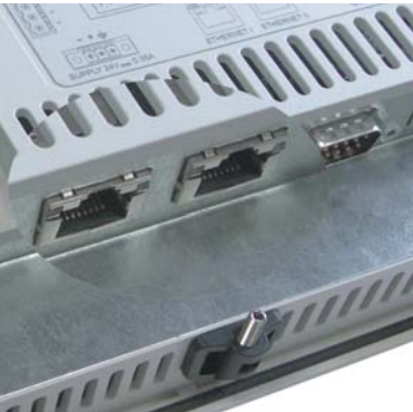
Figure 14: Ethernet I and Ethernet II
