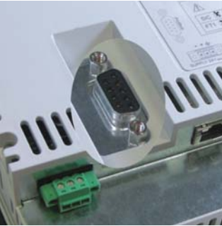
Figure 12: PROFIBUS-DP- SUB-D female connector
