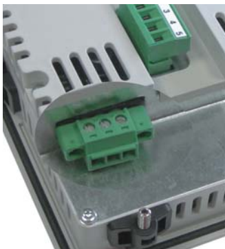
Figure 10: 3-Pin Phoenix Contact- connector
