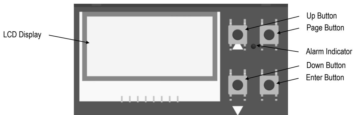
Figure 33: Control Panel for the Comm Box (DIN)
