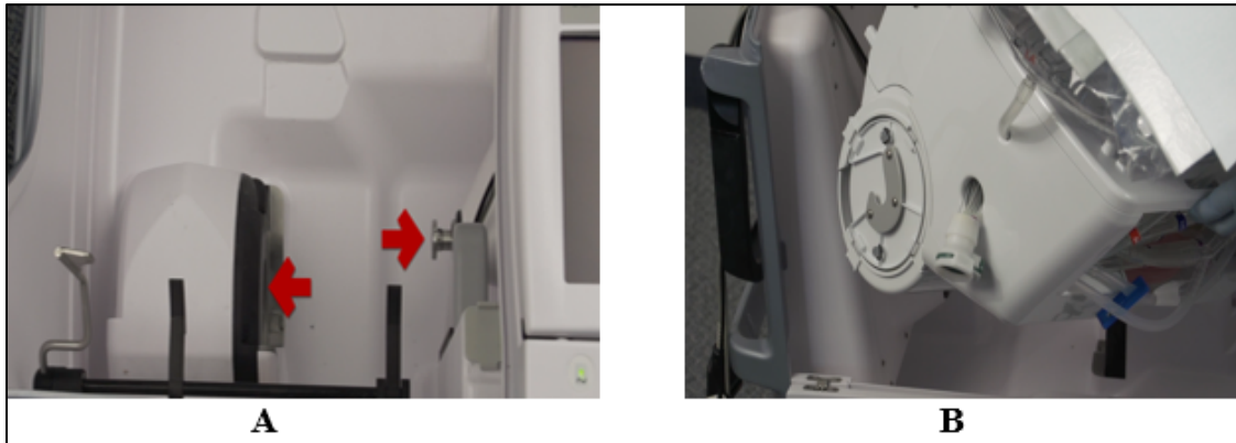
Figure 6: Pump Head, Ventilator Actuator of the OCS™ Lung Console (A) and the Bellows Plate of the LPM (B)
