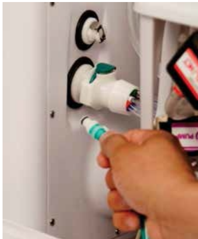
Figure 4-9: Connecting the Monitoring Gas to the OCS™
