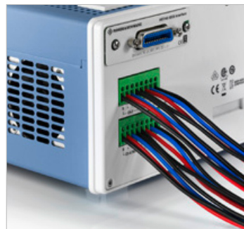
Connections for all channels – including sense lines – are also provided on the rear panel (shown here: R&S®HMP4040 with opt. R&S®HO740 IEEE-488 interface)
