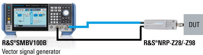
Constant monitoring of signal generator output power and automated level correction using the R&S®NRP-Z28/-Z98 level control sensor
