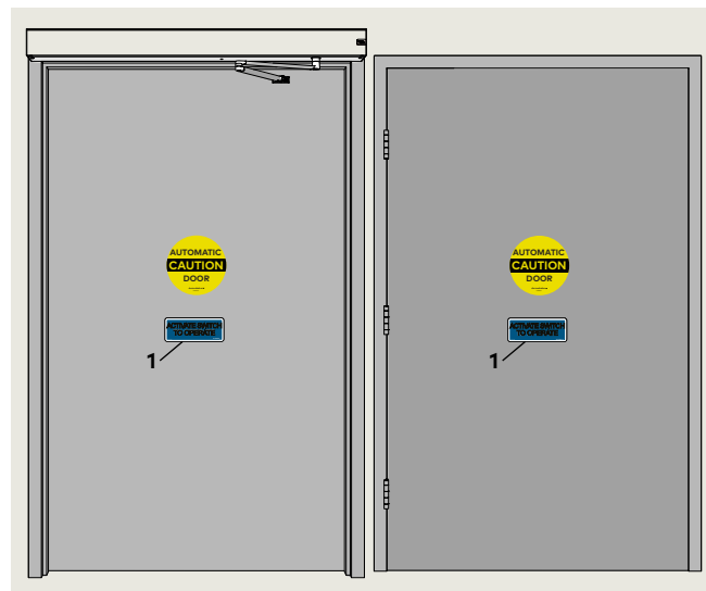
Fig. 11.2.1 Knowing act device initiation of door operation
