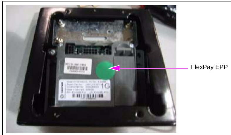
Figure 31: Installing the New Keypad and Screws
