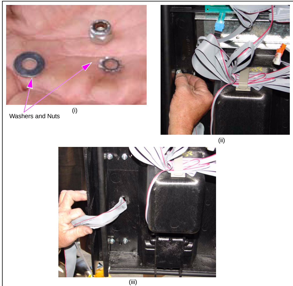
Figure 5: Installing the Washers and Nuts to the Bracket Studs
