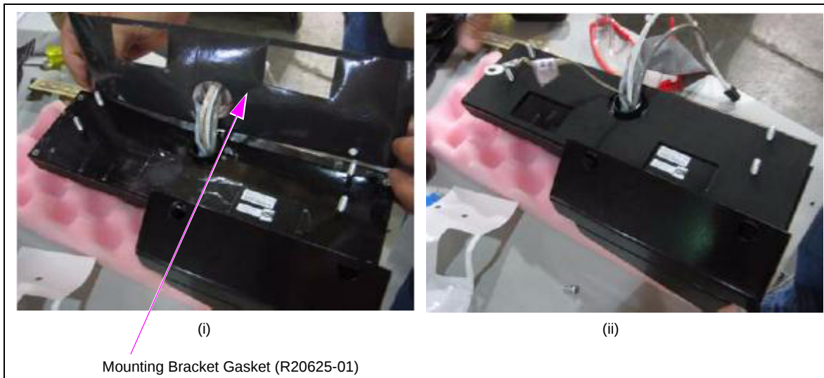
Figure 37: Installing the Mounting Bracket Gasket (R20625-01)
