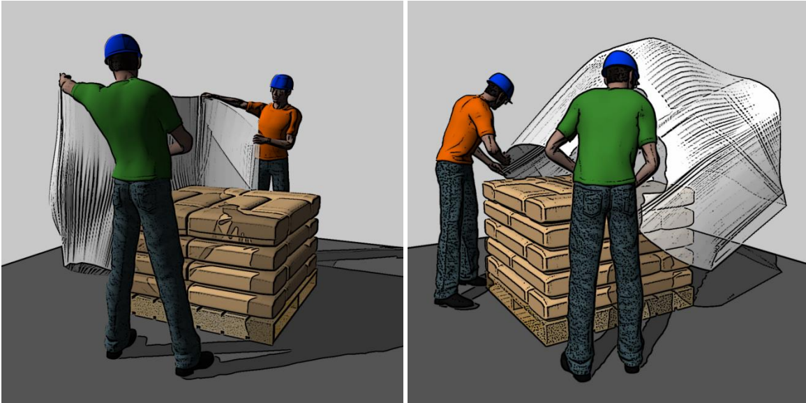
Figure 30. Awkward postures during shrink wrapping: workers' arms are reaching at or above shoulder (left), worker in back is bending and twisting back to the side (right).
