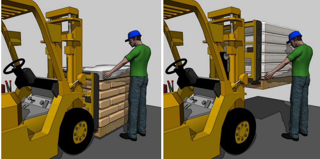
Figure 67. Forklift is used to raise pallet while worker stands still holding corners of shrink wrap. As the pallet is raised, the shrink wrap is pulled down over the stack of bags (beginning of process is shown on left; end is shown on right). As shown, this method does not require awkward reaching with the arms or bending/twisting the back.
