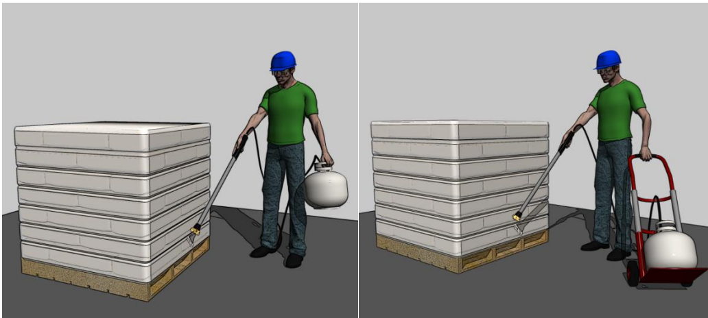
Figure 69. Worker carrying gas tank while shrink wrapping pallets (left). Manual handling is reduced by placing the gas tank on wheeled cart (right).
