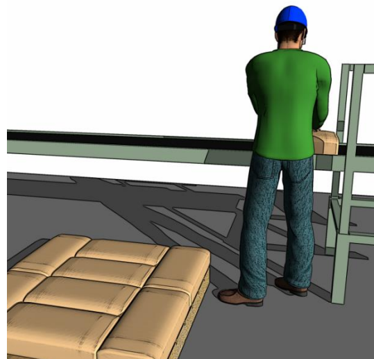
Figure 51. Worker is twisting to the side to pick up a bag from the conveyor belt.
