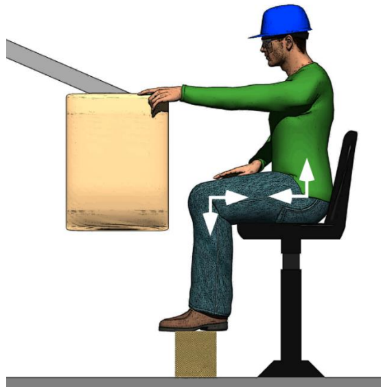
Figure 2. Worker is sitting with hip and knee at same level, hip and knee at approximately 90 degrees, and get supported.
