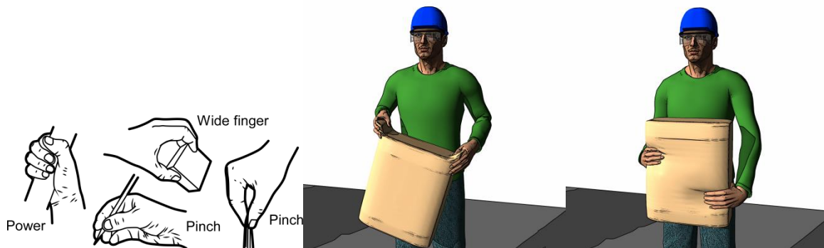
Figure 23. Types of awkward hand grips (left), example of pinch grip when holding a bag (middle), example of a wide finger grip when holding a bag (right).
