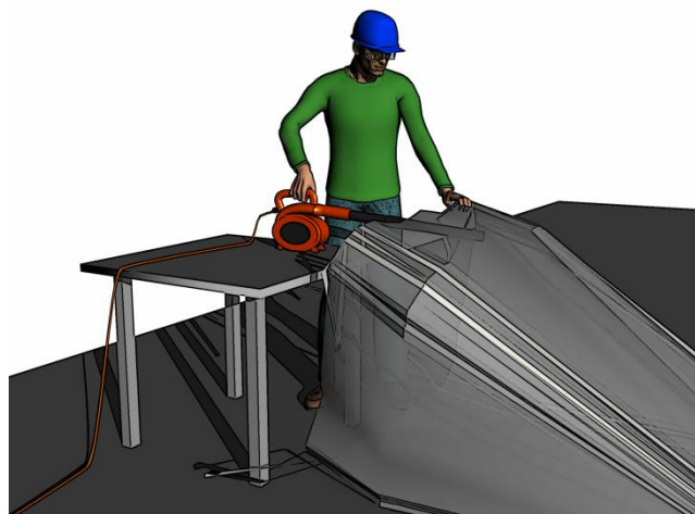
Figure 60. A leaf blower is used to force air into the bag to open it. The leaf blower is supported from beneath and is at a height that allows the worker to control it without bending over.
