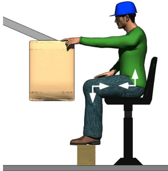
Figure 35. Worker is sitting with the hips and knees at the same level. Both the hips and knees are at approximately 90° angles and the feet are supported.
