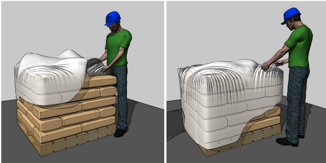
Figure 66. Worker is applying shrink wrap without awkward reaching with the arms or extreme bending/twisting of the back.
