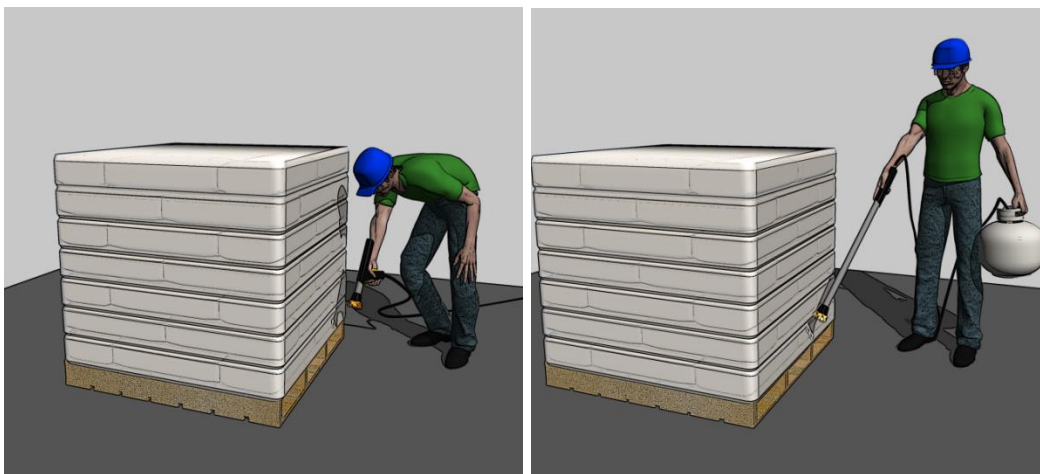
Figure 68. Short wand requires worker to bend forward to reach bottom of pallet (left). Long wand enables worker to reach bottom of pallet without bending forward (right).
