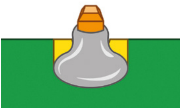
▲ Figure 1-13: A well-soldered pin
