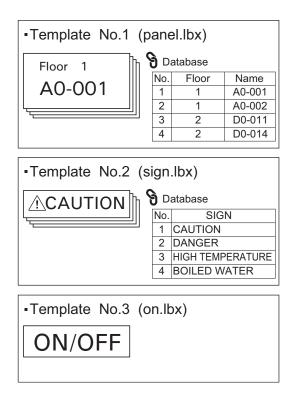
■ If [Template] was set, starting with template number 1, templates are registered with the one-touch key of the same number.
