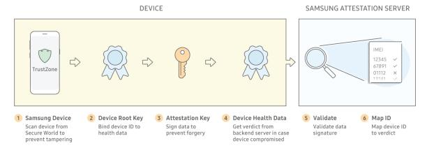
Because a <u>Device Root Key</u> (DRK) is unique to each device, it can tie data to a device through cryptographic signatures. The <u>Samsung Attestation Key</u> (SAK) signs the Attestation data to prove that it originated from the TrustZone Secure World on a Samsung Knox device.
