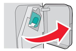
2 Pull the latch of the staple cartridge holder down, and then pull the holder out of the printer.
