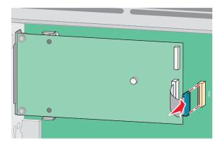
**12** If a printer hard disk was previously installed, then attach the printer hard disk to the ISP. For more information, see <u>"Installing a printer hard disk" on page 29</u>.
