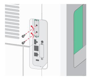
**c** Remove the printer hard disk by pulling it upward to unseat the standoffs.
