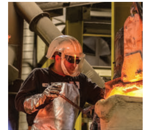
A foundry worker pours liquid bronze into molds.
