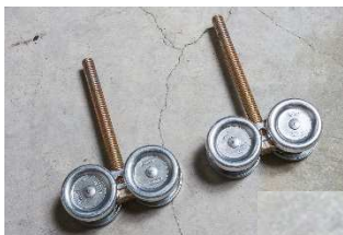
1/2" Bolts shown installed in Roller Assemblies
