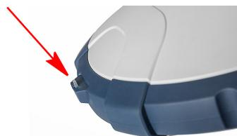
When the receiver is mounted on a tripod – for example – making a slant measurement to determine the instrument height is often more convenient than making a vertical measurement from the ground mark to the antenna base.
