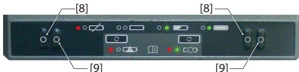
3. Charging the battery will take a few hours. When the battery reaches full charge, the LED ([9]) will turn solid green (see also printed instructions provided with the charger).
