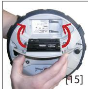
As opposed to previous receiver models, the battery trapdoor of the SP60 can entirely be detached from the receiver case.
