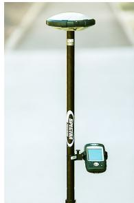
The SP60 has no network connectivity device of its own, but the data collector, to which it is connected over Bluetooth to run the field software, may have this capability (internal modem operated in GPRS mode, using a suitable SIM card). So network corrections received using the data collector modem will be forwarded to the SP60 over Bluetooth as well. In this case of use, the SP60 will be able to deliver RTK positions using one of the following standard network connection types:
