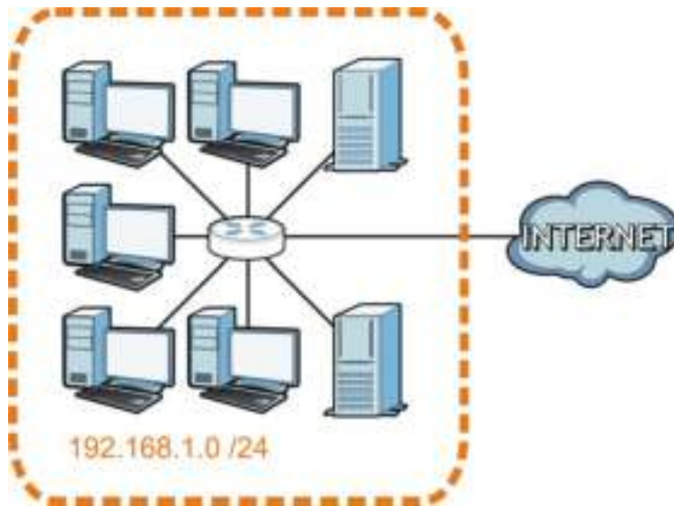
Figure 119 Subnetting Example: Before Subnetting
