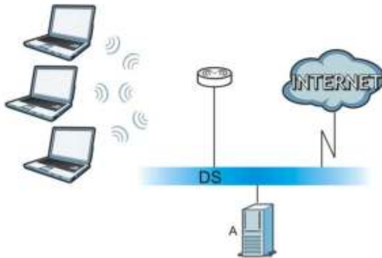
Figure 147 WPA(2) with RADIUS Application Example
