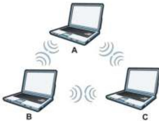
Figure 143 Peer-to-Peer Communication in an Ad-hoc Network
