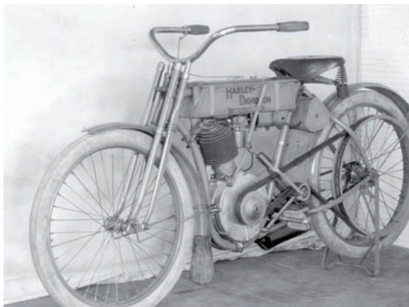
1907 (above) Harley-Davidson motorcycles first started employing spring-suspension front ends – often called ‘cushion forks’. Prior to that, seat springs were a rider’s best defence against bumpy riding conditions.
