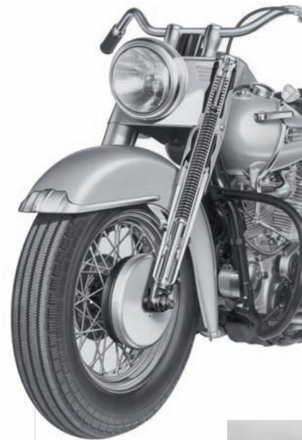
1949 (above) Perhaps the biggest leap forward on the front end of the motorcycle came with the hydraulic front fork introduced on the 1949 Hydra Glide model.
