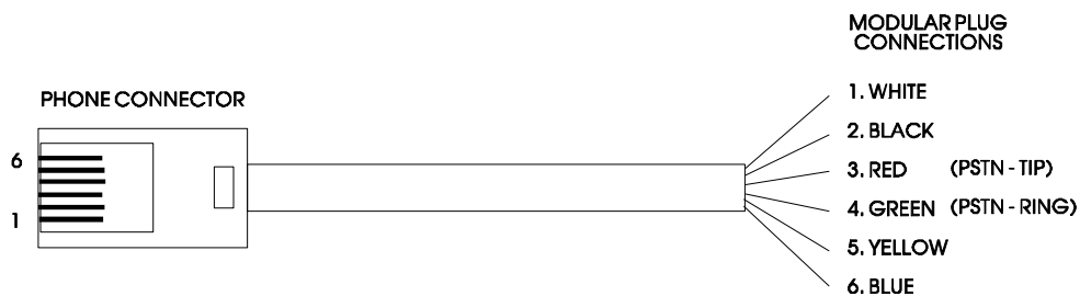
Figure 2-28. Phone Cord Wiring
