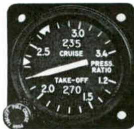
Modern thrustmeter—one of many special Instruments which uses Veeder-Root counting ingenuity—shows pilots the power conditions necessary for safe take-off.
