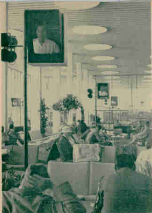
No matter where you are in Copenhagen's new airport building you see on slides, by DISA closed-circuit television, announcements of plane arrivals and departures. You also see and hear the girl who transmits these and other messages
