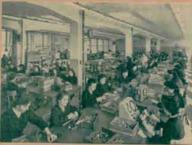
Black-coated girls assemble potentiometers in a Mial plant at Milan. White-coated girls in the Rome plant of a subsidiary make polystyrene capacitors.
