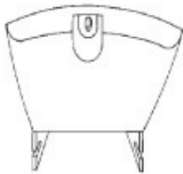
STRAIGHT SIDE SUPPORT Used on the straight side of the pool-notice the square cutout. Use on oval uprights.
