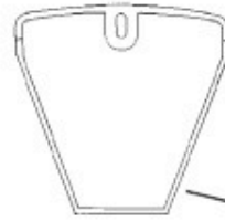
TOP VIEW OF CURVED SIDE ANGLE SUPPORT: Larger than straight side support. Has back wall. Use on curved end uprights.
