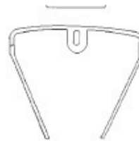
TOP VIEW OF STRAIGHT SIDE SUPPORT: Smaller piece that is open in back. Use on oval uprights.
