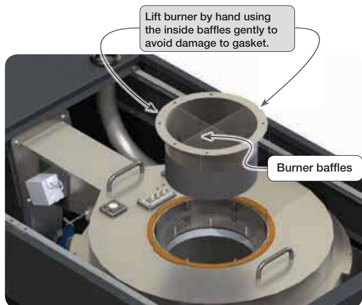
Figure 89 Burner removal and replacement position
