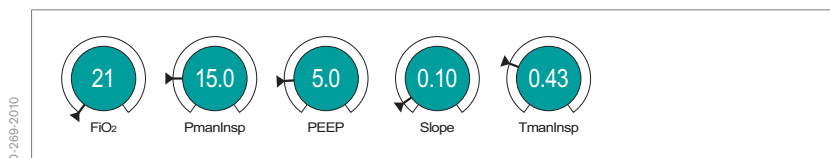
Figure 40: Possible ventilation settings
