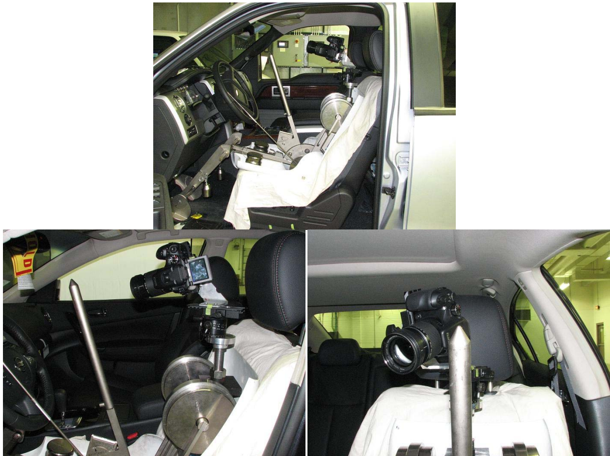
Figure 26. Photos of the Image Quality Assessment Camera Fixture Installed in Test Vehicles
