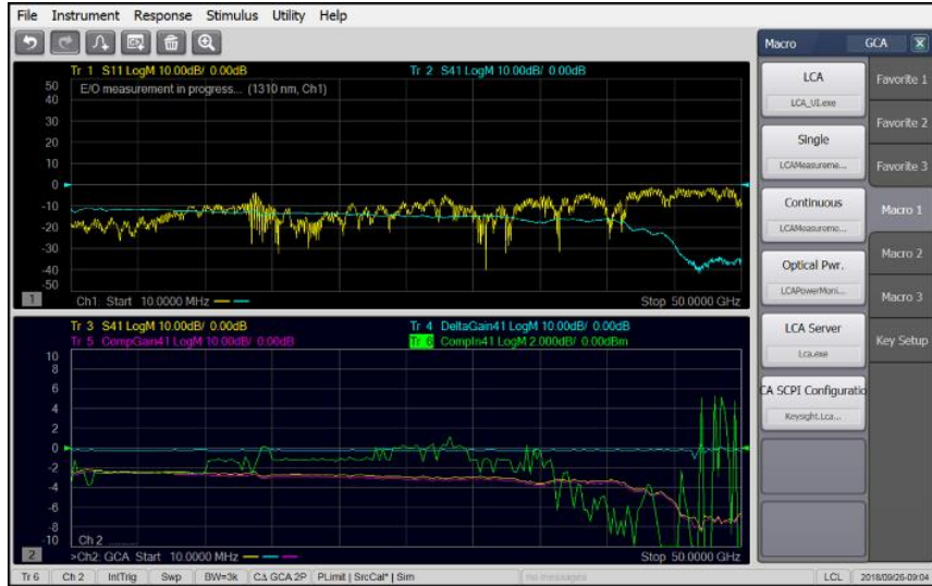
Figure 1: Screen with LCA measurement (upper window) and Gain Compression Measurement (lower window)
