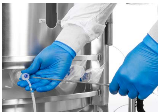
Figur 5–43. Stoppa in temperatursensor.
