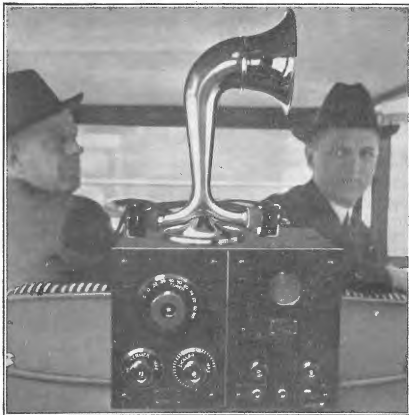
The receiving equipment installed in the car.
