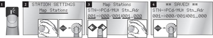
Each station can be mapped to, or associated with, other hardware by way of the 8 numbers to the right of the arrow. The field labeled SS is the Sentinel station to be mapped (01-48). The rest of the fields depend on the Station Type programming (below).
