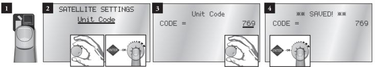
**IMPORTANT:** The unit code is required for Central Control operations. Even if most of the satellite programming will be from the central software, the Unit Code must be set.
