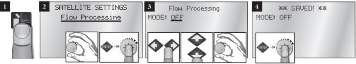
Note: For the controller to read and react to flow, a flow meter must be connected to the satellite sensor terminals. Do not turn on flow processing if it is not properly set up.
