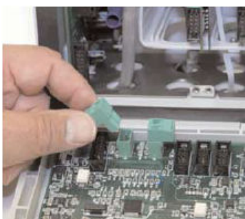
Figure 4-2: Current Output Wiring
