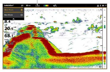
Choose Clear Mode to see less clutter and more fish size accuracy on the display. When Clear Mode is selected, the clutter is filtered, and sonar returns are interpreted to provide more details about the objects within the transducer beam, regardless of their location. In other words, a large arch on the display means a large fish has been detected.
