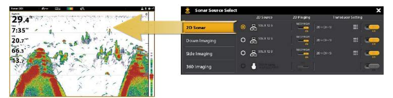
The transducer you select on the Down Imaging tab will provide the data for the Down Imaging Views and related digital readouts.
