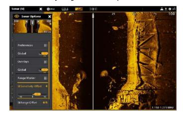
The images you see on the Down Imaging display are produced using sonar technology. Each time the unit pings, a strip of data representing all the echoes received by the transducer are put together on the display to form the image that you see. Like traditional 2D Sonar, the sonar history scrolls left across the screen.
