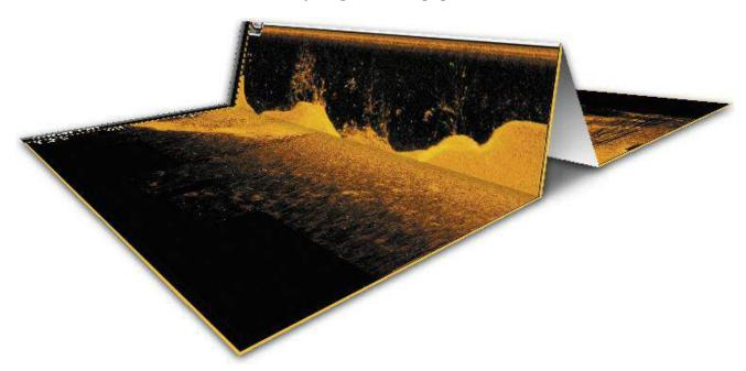
To visualize how Side Imaging works, the Side Imaging View illustration can be folded down the middle and then folded again at the lowest point of the water column. The raised area reveals the water column with its relative depth of the water under the vessel. In the Side Imaging View, variations in the width of the water column show variations in the distance to the bottom as the vessel passes over.
