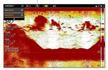
Choose Max Mode to see only raw sonar returns on the display. When Max Mode is selected, you will see the maximum sonar information available within the transducer beam, so more fish arches and better jig tracking are shown.
