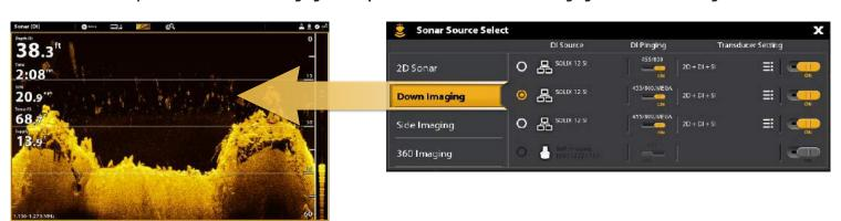
The transducer you select on the Side Imaging tab will provide the data for the Side Imaging Views and related digital readouts.
