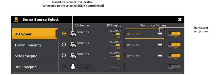
6. **Sonar Capabilities:** On the Transducer Setup menu, add a check mark next to each sonar capability for the selected transducer.
