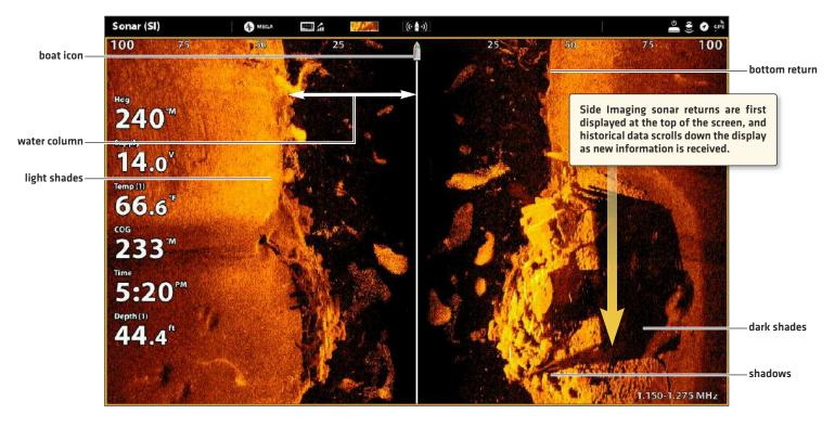
Use the light and dark parts of the display to interpret the objects on the view as follows:
