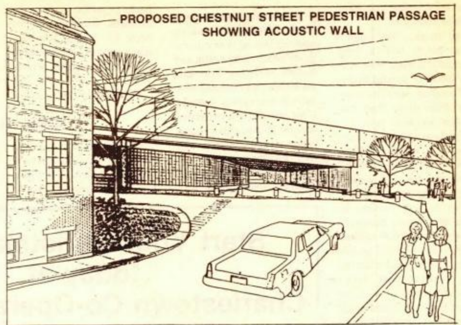
THE ABOVE VIEW is from Chestnut Street, looking through the proposed pedestrian passageway to the water. A solid glass block wall is proposed to protect pedestrians from fumes from the Route 1 south roadway, which pass under this passageway. The Route 1 north roadway would be above the passageway and could include a 12 foot acoustic wall as is pictured. The view below is of the proposed passageway and highways without a 12 foot acoustic wall.
