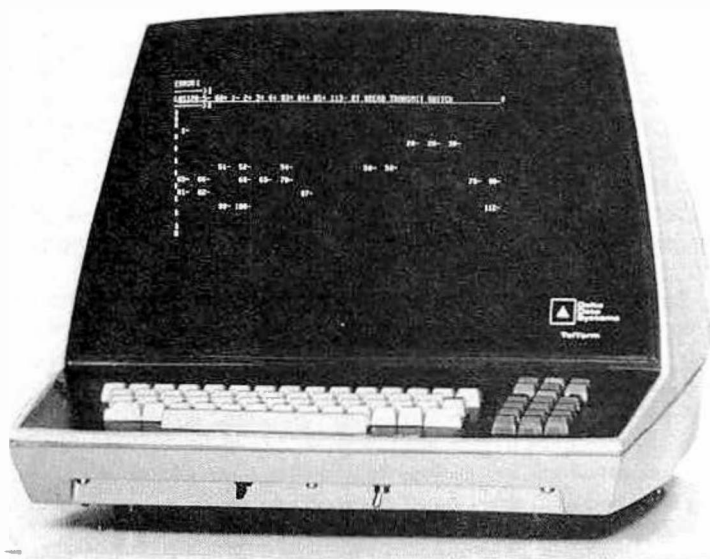
Fig. 23-2. Actual display of faults on the crt of a diagnostic computer.
