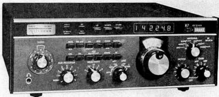
Fig. 10-3. A synthesizer and a permeability tuned oscillator are also used in the Drake R7 receiver (courtesy of R.L. Drake Co.).
