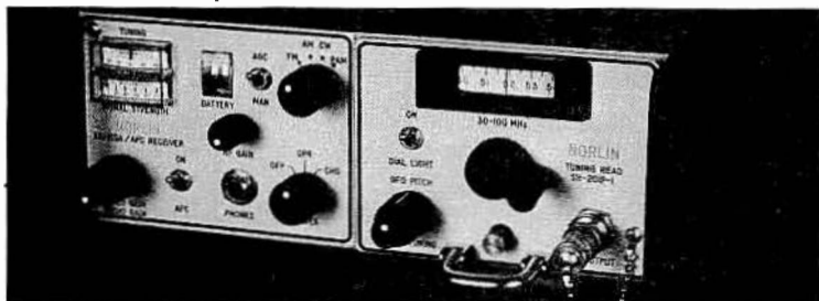
Fig. 13-3. The SR 219 A/AFC receiving system can cover the frequency range of 20 MHz to 4 GHz, with proper rf plug-in tuners. The receiver is used for reception of AM, FM, cw and pulse signals and can be operated as a fixed or portable unit (courtesy of Norlin Communications).
