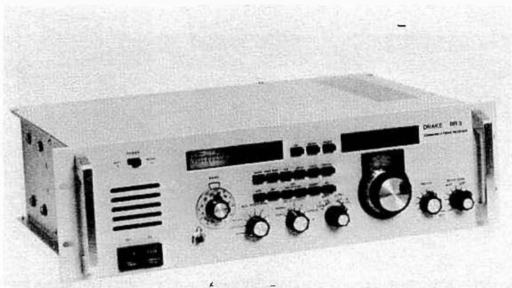
Fig. 10-1. The RR 3 communications receiver is a modern implementation of a triple conversion approach with the first i-f at 48.05 MHz, the second i-f at 5.645 MHz, and the third i-f at 50 kHz. This receiver was designed primarily for maritime communications (courtesy of R.L. Drake Co.).
