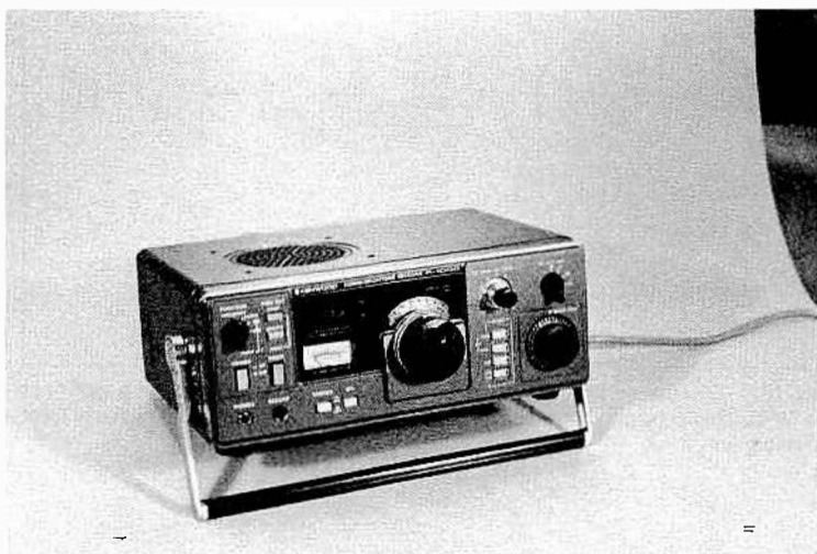
Fig. 10-1. The RR 3 communications receiver is a modern implementation of a triple conversion approach with the first i-f at 48.05 MHz, the second i-f at 5.645 MHz, and the third i-f at 50 kHz. This receiver was designed primarily for maritime communications (courtesy of R.L. Drake Co.).
