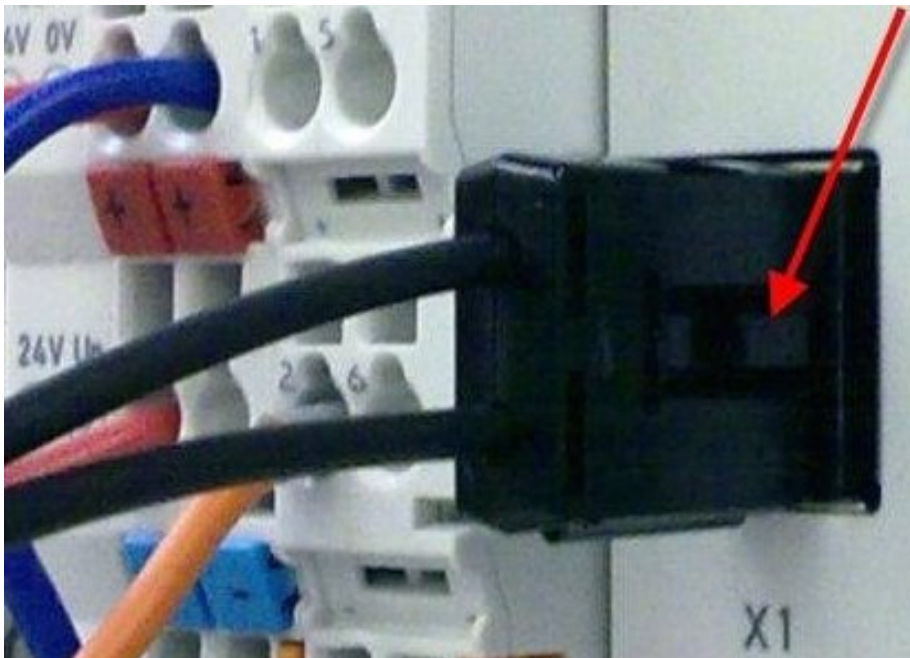
Fig. 32: Latching lug with release catch on the POF duplex plug
