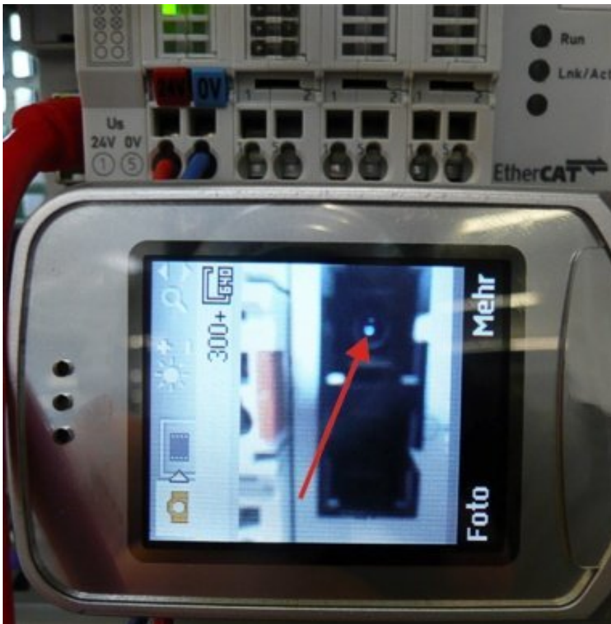
Fig. 30: Visualization of infrared light at the SC duplex connector
