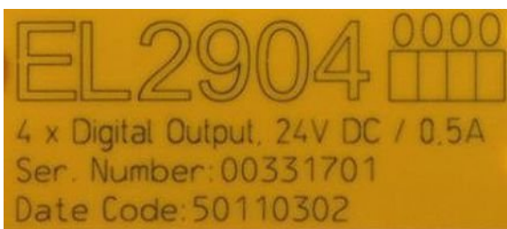
Fig. 7: EL2904 IP20 safety terminal with batch number/ date code 50110302 and unique serial number 00331701
