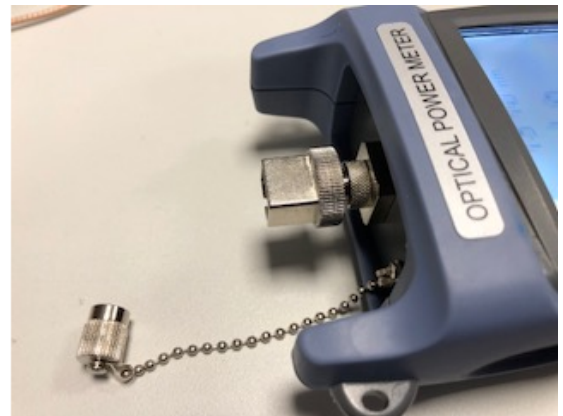
OPM with FC and SC adapter screwed on - WRONG
