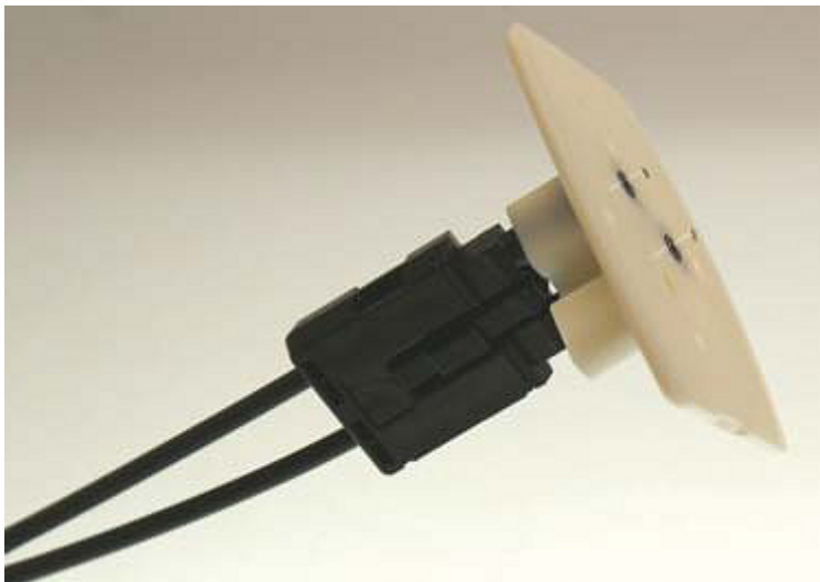
Fig. 40: Sanding gauge with protruding fiber ends
