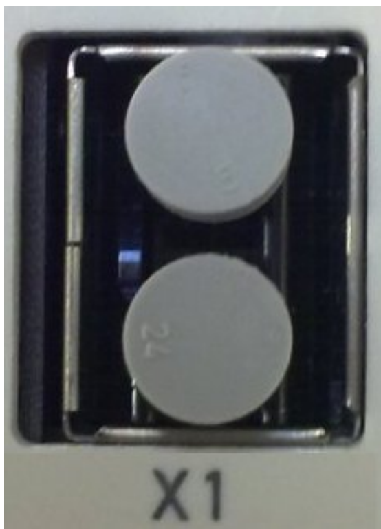
Fig. 34: Blind plugs in unused sockets
