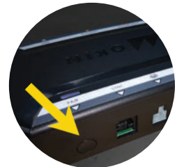
Pairing method 2: Press the PAIR button twice.
