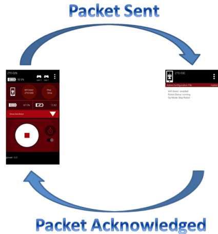
Figure 29 - Ping time represents the time it takes for a packet to be sent to and acknowledged by the Robot Controller.
