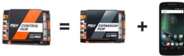
Figure 3 - A Control Hub is a Robot Controller with an internal Android device.
