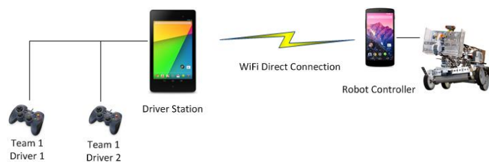
Figure 1 – Each DS-RC pair has its own unique wireless connection.
