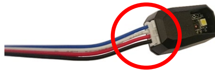
Figure 49 - The base of the JST cable is poorly insulated and an electrostatic discharge can occur in this area.
