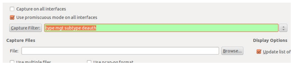
Figure 79 - Specify the capture filter "type mgt subtype death" in the text box.
