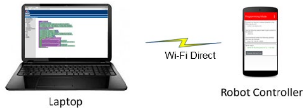
Figure 5 – A team might also have a developer’s laptop connected when they are away from the competition field.
