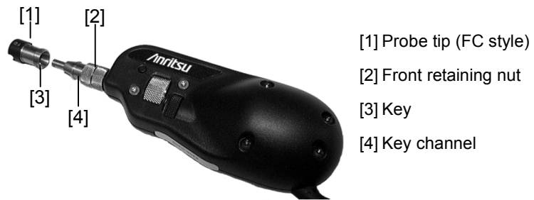
Figure 9.2-2 Attaching a Probe Tip
