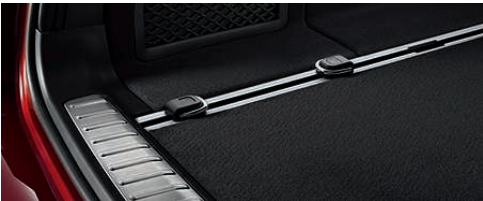
Storage package enhances safety and convenience by securing items of various sizes and shapes during transport. Includes luggage nets on the back of the front seats, under the center console on the passenger side, and on the left side of the cargo area; two cargo rails with four fastening points in the cargo area floor; a reversible mat; multi-purpose hooks; and a tensioning strap.
