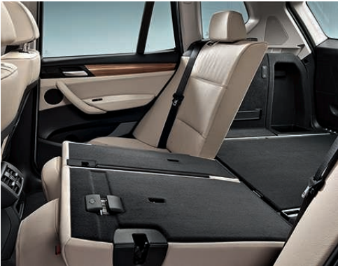
Rear-seat backrests can be divided into a 40/60 split to optimize the number of passengers and amount of cargo. For example, up to four pairs of skis or three snowboards can be carried while still retaining seating space for up to four adults. Rear-seat backrests providing a 40/20/40 split (not shown) afford even greater versatility by providing additional passenger seating and cargo-transporting options.
