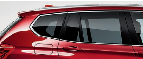
Privacy glass in the rear cabin windows helps suppress excessive heating of the interior and also filters the sun's harmful UV rays more effectively than clear glass.
