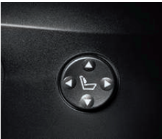
Lumbar support for driver and front passenger seat adds four-way adjustable comfort for the lower back. Lumbar support can be adjusted up/down and in/out.
