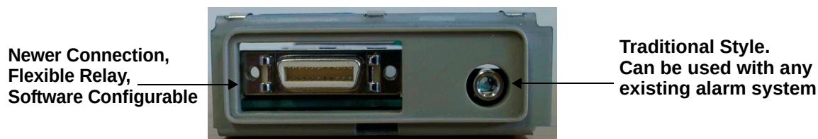
Figure 29 Flexible Nurse Call Relay Connections at Monitor
