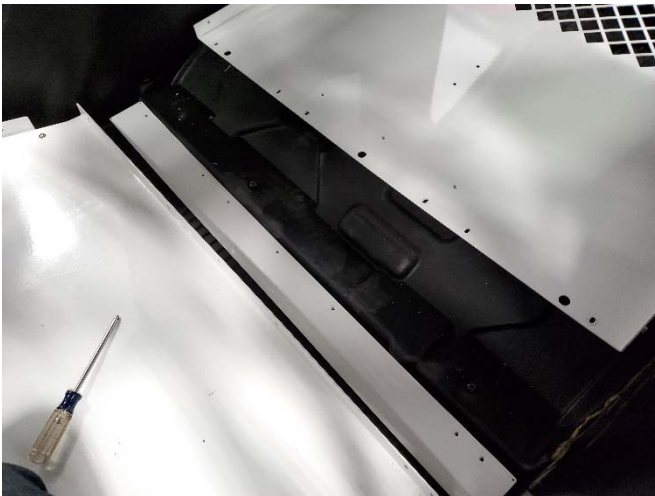
Attach rear cargo filler plate to rear of K9 floor prior to installing rear bulkhead.
