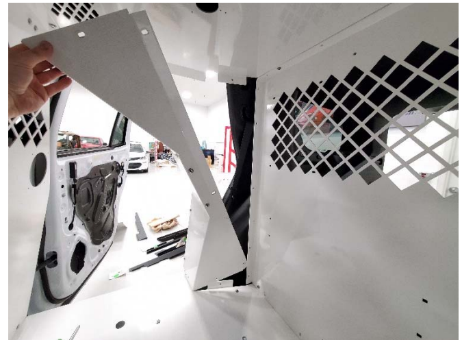
Pre-assemble side trim panels outside of the vehicle. Place inside as one piece.
