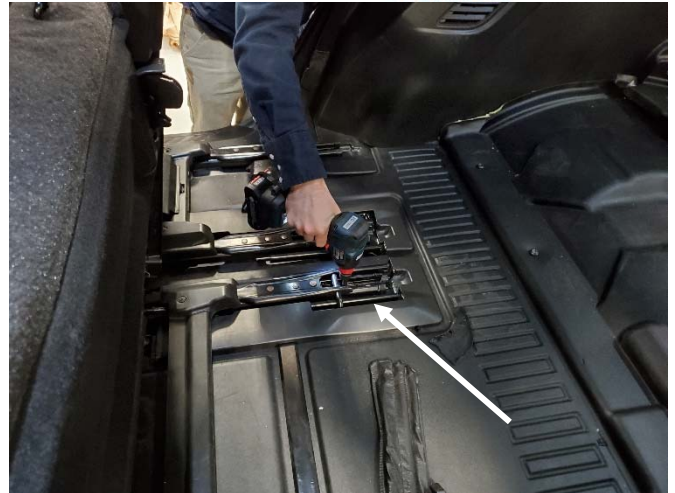
Flip seat seats forward to access hardware.
