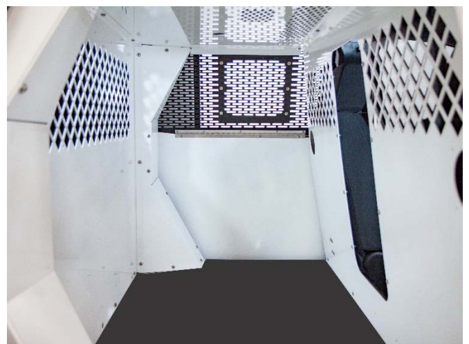
After silicone is dry, place in rubber mat to complete installation.
