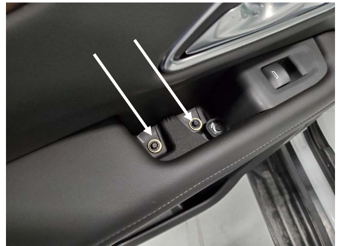
Remove plastic covers behind armrest handle. Remove screws. (7mm socket) Note: A small 90° scribe helps to pick plastic covers off.
