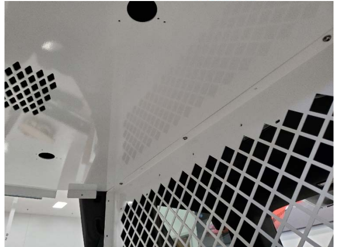
Place ceiling panel on top of front and rear bulkheads.
