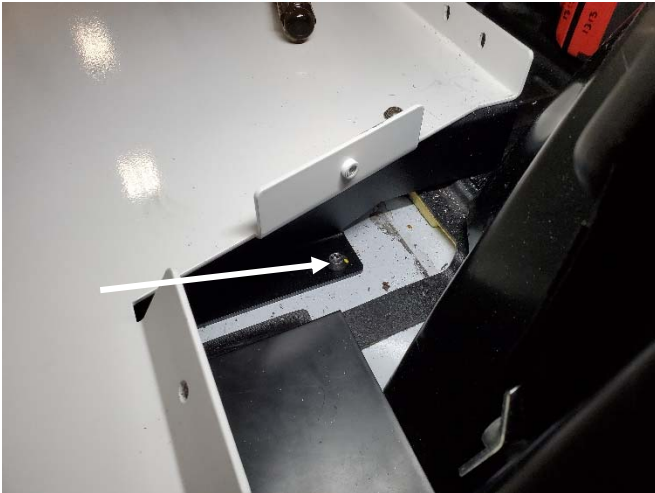
Tighten rear floor mounting hardware.
