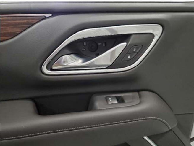
Remove plastic covers behind the paddle handle. Remove screws. (7mm socket) Note: A small 90° scribe helps to pick plastic covers off.
