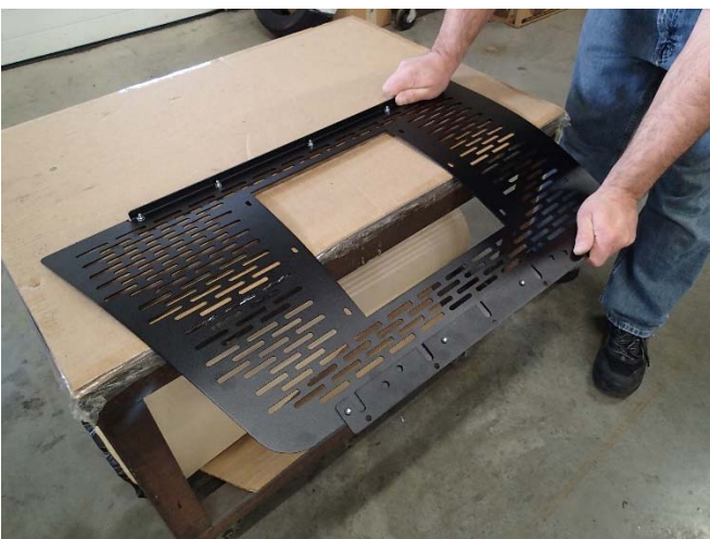
NOTE: Window guards are shipped flat. On the edge of a workbench, bend a contour in the middle of the guard so it will fit tight against the window frame.
