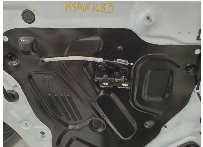
Remove / unsnap entire door panel from door. (Trim removal tool) Remove armrest bracket.
