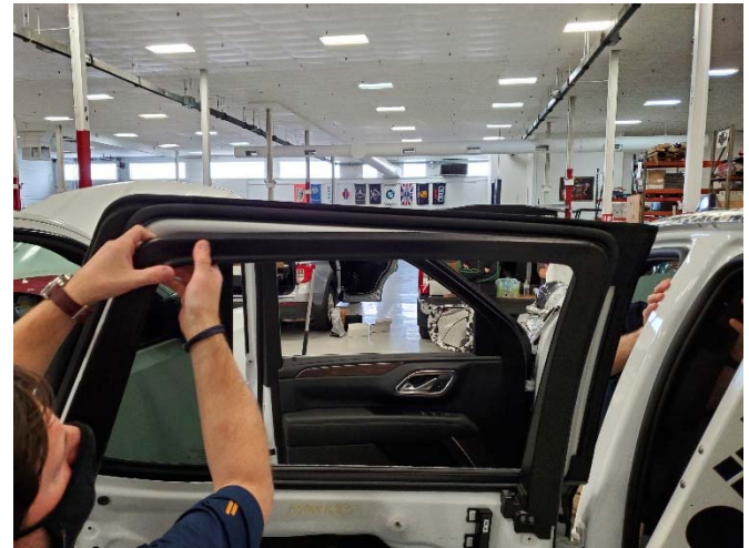
Gently remove trim around window frame.
