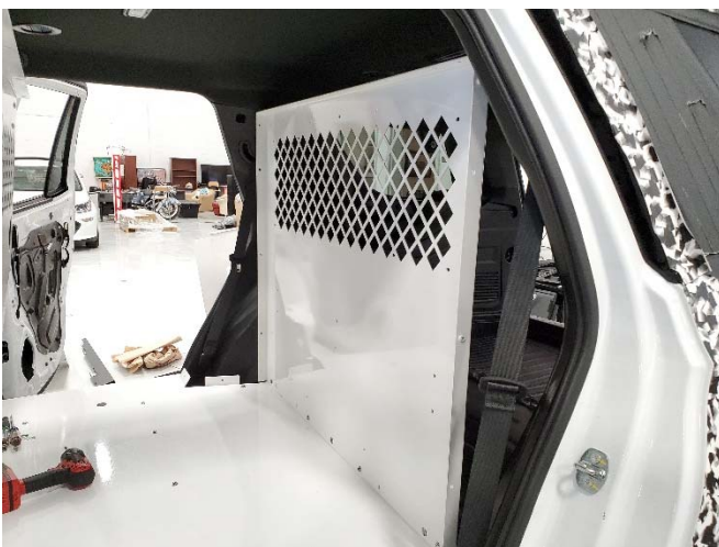
Attach rear bulkhead to floor using 1/4" x 3/4" Phillips head bolts and flat washers.
