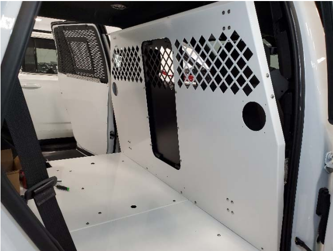
Attach front bulkhead to floor and B pillar mounting brackets with 1/4"x 3/4" carriage bolts and nuts.
