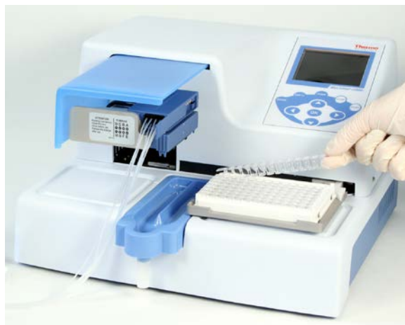
Figure 6–49. Removing the filled microstrip to be weighed
