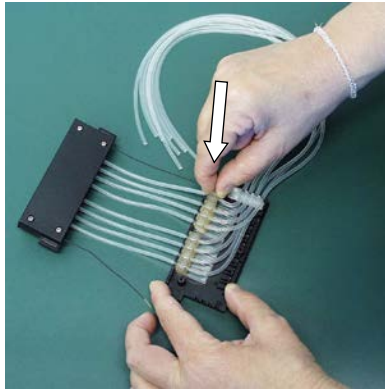
Figure 5-37. Pressing the tube fasteners into place
