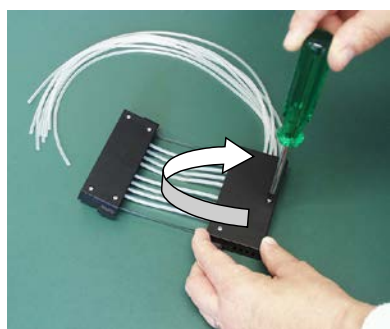
Figure 5-42. Fastening the cover retaining screws
