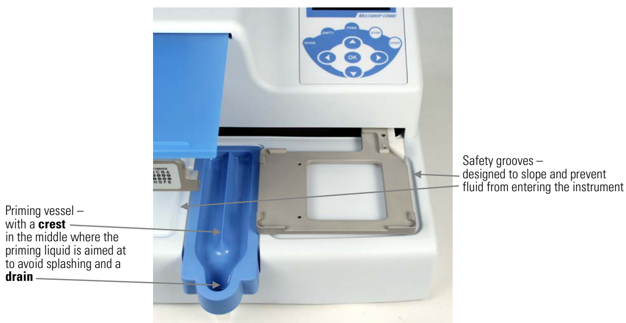
Figure 4–9. Priming vessel inserted into place
