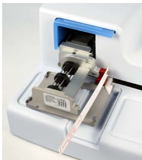
Figure 3–5. Transport lock and transport lock tag present
