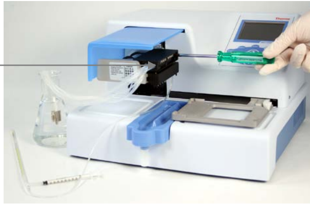
Figure 6–51. Screwing the calibration screws according to the calibration results
