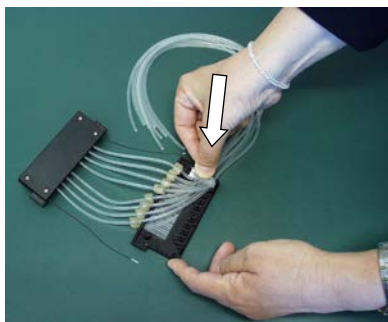
Figure 5-36. Pressing the tubing identification plate into place
