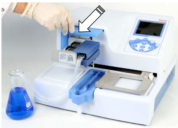
Figure 4–20. Pulling the rotor cover over the rotor
