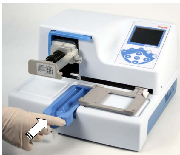
Figure 3–8. Inserting the priming vessel
