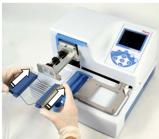
Figure 4–11. Inserting the dispensing cassette
