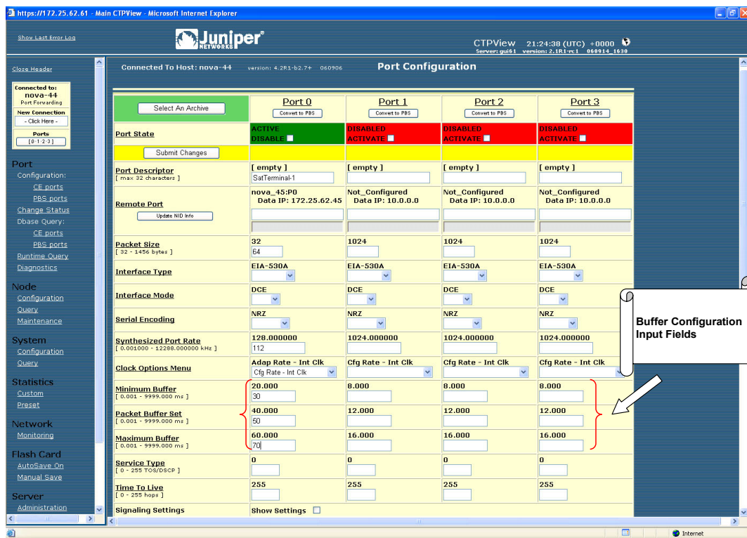
Figure 46: CTPView Receive Buffer Fields
